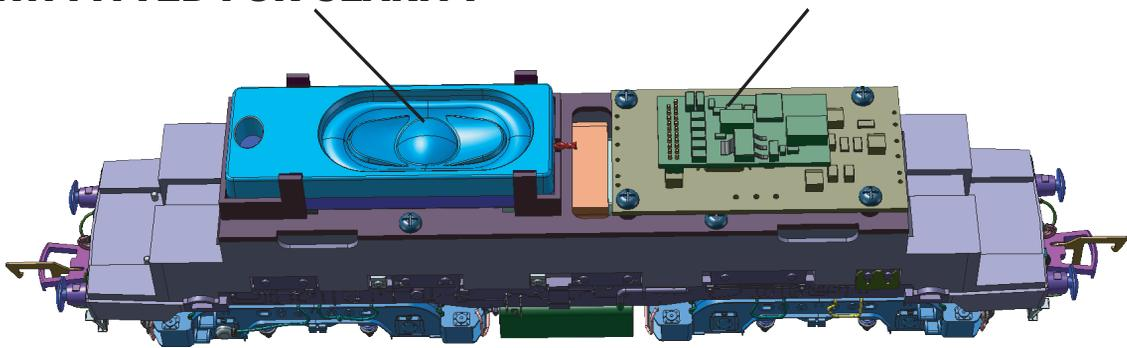
To fit a DCC decoder (please remember that your model will work normally on DC straight from the box upon purchase), please refer to the simple picture graphic within the pages of these instructions showing the DC (normal operation) blanking plug that needs to be exchanged for the DCC 21 pin decoder of your choice. The location of the simple clip in speaker is also shown for clarity.
