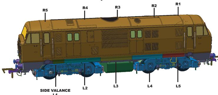
Upon removal of the body these may fall out, but please do not worry as that is a design feature not a fault, and they will simply clip back in between the body and chassis. It is suggested that if you wish not to use all the valances or have some missing, which is very prototypical, that you keep them stored within the locomotive box. Dapol will stock spare valances, but this may be some time after the initial models' release.
