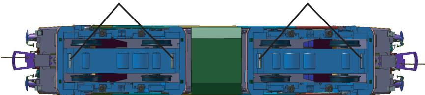
To oil the motor worm bearing just remove the body (unplug this from the chassis) and add 1 or 2 small drops of oil to the circular metal piece at the end of the bogie.
